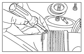
1. Unscrew the clamp on the air duct hose.
